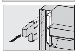
Fit the wall spacers onto the back of the appliance on the top left and right.
